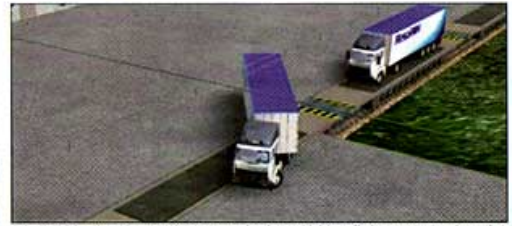
RésoR@il loading schematic. (Note: tractor heads would drive off after positioning the trailer)
